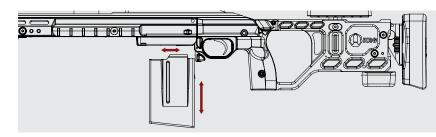
**Step 2:** Push in on the thumbscrew to disengage the LOP lock.
