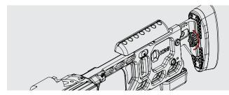
**Step 2:** Slide the buttpad up or down in 1/4" increments, or cant it 15 degrees to either side. There are protrusions on the aluminum LOP bar that fit into pockets on the polymer buttpad housing. Retighten Thumbscrew when you have it set where you want.
