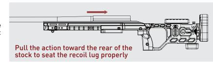
**Step 5**: Making sure the action is level and not canted to the left or right, next tighten all three action screws until they are snug but not fully tightened.
