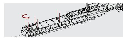
**Step 3:** If unable to achieve desired fit, trigger guard can be moved forward and backward a small amount as well. Remove action from stock, loosen screw holding trigger guard to stock, reposition trigger guard, re-tighten screw.
