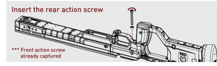
**Step 4:** Pull the action towards the rear of the stock while holding the stock stationary. This is to seat the action against the recoil lug. A good way is to set the rifle vertical on the buttpad and bounce it lightly on the ground a couple times.
