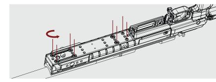
**Step 2:** Slide the forend forward or backward a small amount to achieve the desired fit of the magazine into the stock. Re-tighten screws from step 1.
