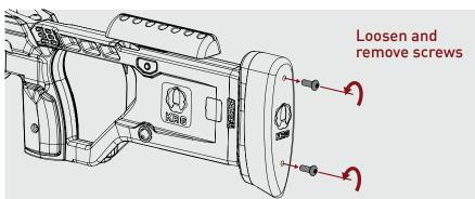
**Step 2:** Replace these screws with the longer screws, which are long enough to go through your desired amount of spacers. Insert desired quantity of spacers onto the longer screws
